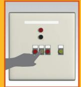
The Salvo SGL is placed over the emergency airline coupling releasing the trapped Salvo key and locking the Salvo SGL on. The trailer brakes are locked on. The Salvo key is then taken back to the Salvo Control Panel (SCP) at the loading bay.
