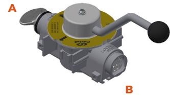
Key A stays trapped and key B is released while the valve locked closed.
