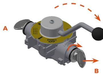
By inserting and turning key A in the MBV, the valve can be released from locked open condition and changed to closed. By turning and releasing the key B the valve is locked in the closed condition.
