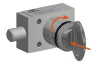
Inserting and turning the key retracts the bolt against the spring load. This will trap the key into the lock. The key must be held in this position until bolt movement is inhibited by the mechanism. 3 Key is trapped, bolt is retracted
