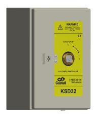
The KSD is a key driven non fused switch disconnector for the isolation or switching of currents. The standard KSD comes with 4 or 6 poles plus 2 auxiliary early break contacts. The KSD is manufactured from either brass or stainless steel. The unit is supplied suitable for mounting into an existing panel or for surface mounting within its own IP65 rated lockable mild steel enclosure.
