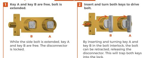
Keys are trapped, bolt is retracted.
