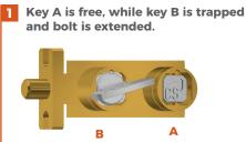
While the side bolt is extended and key B is trapped, key A is free. The disconnector is locked by the extended bolt of the KLF. 2 Insert and turn key A, then turn key B to drive bolt, releasing key B.
