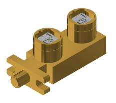
The KLF Lock is a multi-key operated mechanical bolt interlock for the control of electrical switchgear. The standard unit comes with a 16 mm diameter bolt of variable length, that is used to control the rotation or movement of operating handles or toggles of electrical switchgear. This lock is manufactured in brass or stainless steel. The KLF bolt interlock is available in a double key or exchange key condition.
