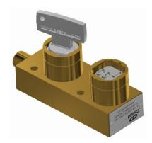
The KL Dual Key Bolt Interlock is a key operated mechanical bolt interlock suitable for the control of electrical switchgear. The interlock is used to control the rotation or movement of operating handles or toggles of electrical switchgear and is manufactured in brass or stainless steel. The KL Bolt Interlock is available in a double key or exchange key condition.
