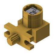
The KF Lock is a key operated mechanical bolt interlock for the control of electrical switchgear. The standard unit comes with a 16 mm diameter bolt of variable length, that is used to control the rotation or movement of operating handles or toggles of electrical switchgear. This lock is manufactured in brass or stainless steel.
