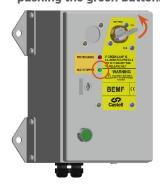
Turn the key to OFF position to switch the power off. A movement detector gives a signal to the BEMF unit once zero movement has been detected. This will illuminate a green LED. The key may now be released by pushing the green button. This key is then taken to unlock the access lock on the motor unit.
