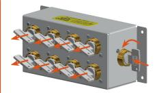
By inserting and turning the free end key in the Y key exchange box, you can release the trapped front keys in any order. Once the first key has been removed, the end key stays trapped. The released keys can be used in the access door locks to gain access to the hazardous area. End key is trapped, front keys are free
