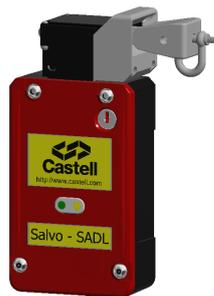
To open the guard the machine is instructed to stop via control circuit. On stopping a signal is sent to the solenoid in the OLYMPUS unit. With the solenoid energised, the tongue actuator can be retracted to break the contacts ensuring the machine cannot restart.
