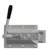
Under normal operating conditions, the isolation key is free, the personnel key is trapped, the catch is retained and the door is locked closed. Insert and turn isolation key, then release personnel key and release catch from locking mechanism by operating the handle.
