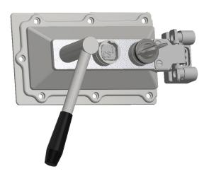
The EDIX is a key access interlock complete with emergency exit system for use on hinged doors. The interlock is manufactured in durable stainless steel and comes with the stainless steel FS or Q lock type portions. Two internal crashbar options are available: a light duty two point aluminium and a heavy duty three point stainless steel. Typical industries using the EDIX are fire protection, turbine and offshore industry.
