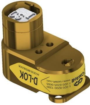
The D type lock is a two-part interlock, comprising of a lock body and rear or front entry mounted catch. Typically, the D lock is used for interlocking electrical control cubicles and distribution panels. It is also suitable for use on light access doors or hatches. The catch is available in two options, one suited to well aligned doors, the other suited to misaligned doors. The D lock is available as FS (figure symbol) or Q lock type.
