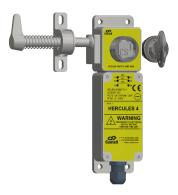
The AIS is a single key access interlock complete with electrical contacts for use on hinged doors. The AIS contacts can be used to switch off the machine via its control circuitry or to initialize a signal to visual beacons/ sounders. The switch is sealed to IP65 with, 1N/O 2N/C contacts, rated to 10 A making it ideal for use in cross monitored safety systems. The interlock is manufactured in a durable stainless steel.
