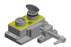
The AIE-HD is a Heavy Duty (HD) robust dual key access interlock that is suitable for use on hinged and sliding doors. The interlock has an open cavity design and is manufactured in stainless steel. The AIE-HD is available in two options: exchange key and double key.
