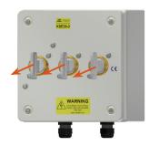
By turning the keys, the contact condition changes switching the power off. The keys can now be released and taken by the personnel to unlock the doors in the machine area. Power is off, all keys are sequentially released
