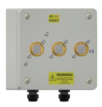
The KSE is a multi-key controlled electrical switch designed for machine control circuits. This type of isolator should be used for short term, off load isolation. The unit is supplied for mounting into an existing panel or for surface mounting within its own IP65 rated lockable steel enclosure. It is available in FS or Q type lock portions. The KSE is manufactured from either brass or stainless steel.
