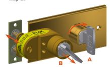
Inserting and turning key A in the bolt interlock enables the release of key B and the release of the catch. This will trap key A into the lock.
