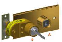
While the catch is trapped in the mechanism, key B is trapped and key A is free. The door is locked closed through the trapped catch.
