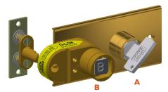
Key B is used as the personnel key and taken to the machine area. Key A stays trapped as long the catch is released and key B is free.
